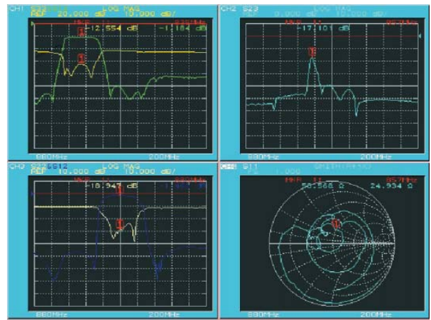
Simultaneous Display of Tx, Rx Isolation characteristics for Duplexer
